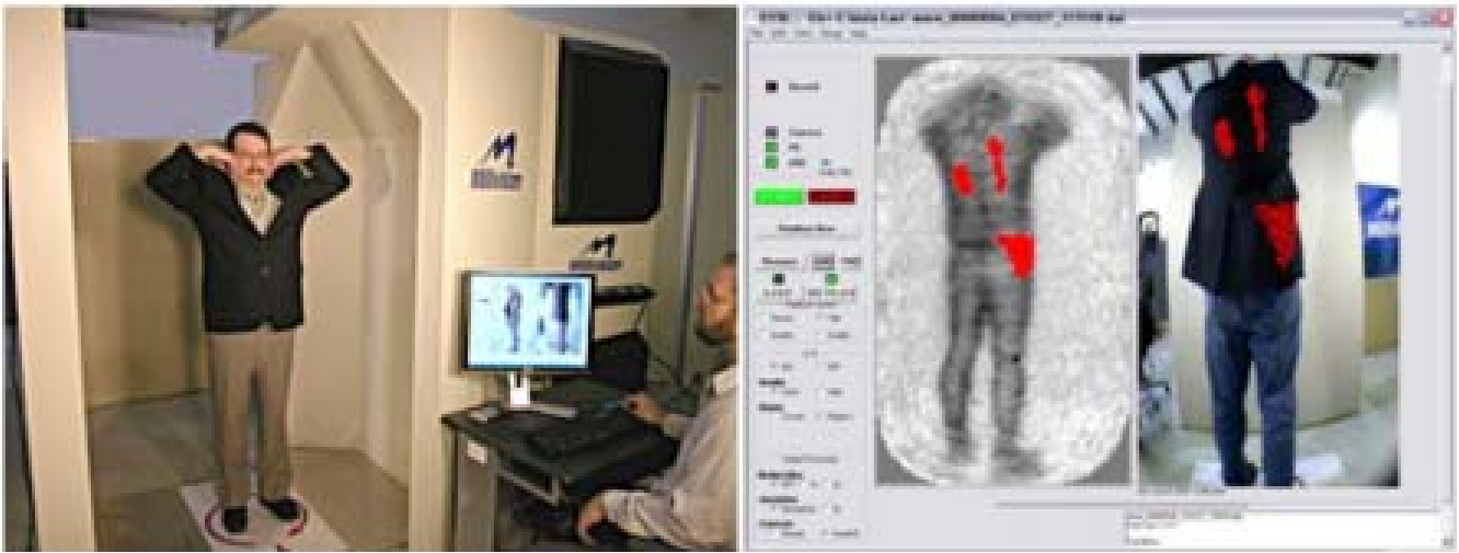
Figure 1. Millivision Portal Systems 350 scanner. On the Right, Screen Display Where ATD Software Enhances Threat items.
